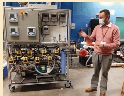
Fig. 1. Student demonstrating a high recovery reverse osmosis pilot unit
